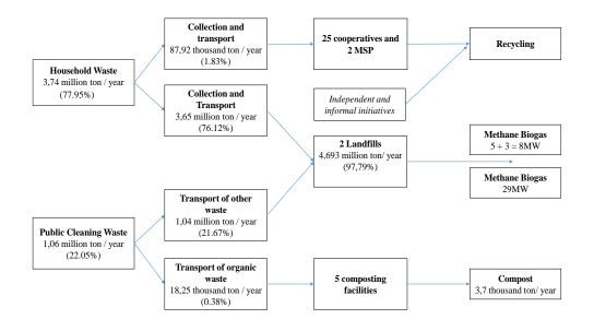
**Figure 1:** MSWMS of the São Paulo city and the quantities of MSW Generated and Managed in 2017.*MSP: Mechanized Sorting Plants.*
